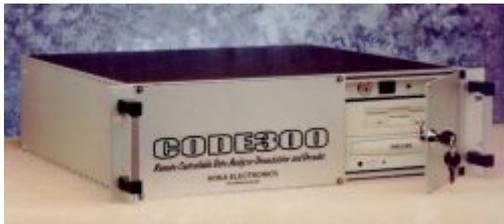
CODE300-A does use the same fairly inexpensive hardware as CODE30-A, but is delivered completely in a 19" rack PC, containing a Pentium 200 MMX, 16 MB RAM and a harddisk with 2.0 GB, Sound Card, SVGA 3D or ET4000, operative system MS DOS and AT-keyboard.
