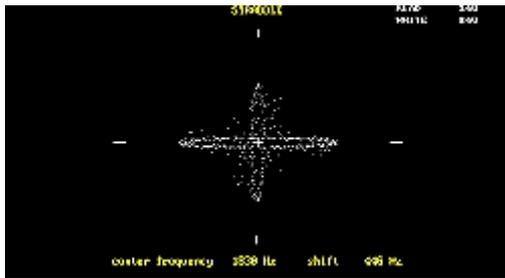
Straddle showing a tuned RTTY signal
