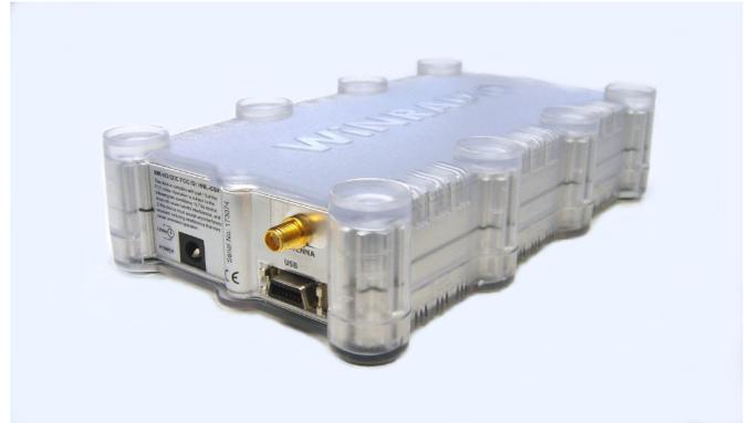
The WinRADiO WR-G31DDC 'Excalibur' is a high-performance, low-cost, direct-sampling, software-defined, shortwave receiver with a frequency range from 9 kHz to 50 MHz. It includes a real-time 50 MHz-wide spectrum analyzer and 2 MHz-wide instantaneous bandwidth available for recording, demodulation and further digital processing.
