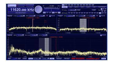
The receiver's superior performance results from its innovative, direct-sampling, digital down-conversion architecture along with the use of leading-edge components and design concepts. These all result in a very high IP3, wide dynamic range, high sensitivity, and accurate tuning. These key features create a receiver in a class of its own, with wide application potential, at a very affordable price.
