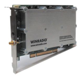
The WiNRADiO WR-G313i receiver is a software-defined high-performance HF receiver (9 kHz to 30 MHz, optionally extendable to 180 MHz) on a PCI card. The front-end is a DDS-based double-conversion superhet, the last IF stage is implemented in software resident in the on-board DSP.
