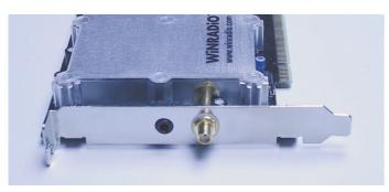
The receiver has its own on-board DSP, and does not rely on the PC sound card for its performance. As the DSP performs the final stage IF filtering and all demodulation, this receiver is entirely software-defined, which means that additional demodulation or decoding modes can easily be added by a mere software change.
