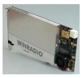
The receiver is very well shielded against interference, making it possible to operate in a noisy computer environment. The receiver card has very modest power requirements of less than 10 watts, allowing it to be powered from the PC's internal power supply. There is also provision for an external power supply feed in cases where several of these receiver cards are to be installed in a multi-channel configuration.
