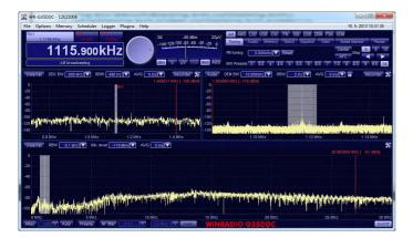
The receiver's superior performance results from its innovative, direct-sampling, digital down-conversion architecture along with the use of leading-edge components and design concepts. These all result in a very high IP3, wide dynamic range, high sensitivity, and accurate tuning. These key features create a receiver in a class of its own, with wide application potential, with many operational and instrumentation features not usually found on receivers of any price category.
