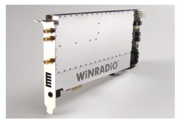
The entire 32 MHz DDC (digitally down-converted) bandwidth is available for recording and demodulation. Multiple demodulators allow the simultaneous reception and decoding of radio signals within the entire HF band.
